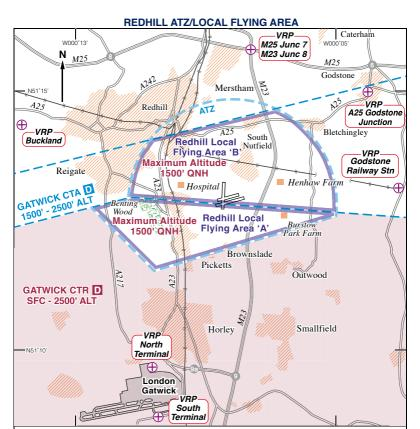
The southern half of Redhill Aerodrome lies within the Gatwick CTR and the northern half lies beneath the Gatwick CTA. During the hours of watch of Redhill ATC, VFR & SVFR flights, without reference to Gatwick ATC, may be made within the LFA subject to compliance with the following restrictions and procedures:
